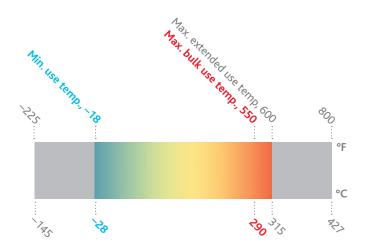
Eastman Therminol® 55 heat transfer fluid is a unique, synthetic fluid designed to provide reliable, consistent heat transfer performance over a long life at maximum bulk temperatures up to 290°C (550°F).
